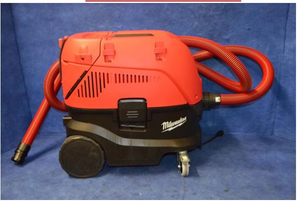
Under contract with Milwaukee tools Inc., LMS Technologies tested HEPA-VAC unit Model number 8960-20 with Fleece Bag Model number 49-90-1955, Main Filter Model number 49-90-1953 and HEPA Filter Model number 49-90-1952 for HEPA Performance.
